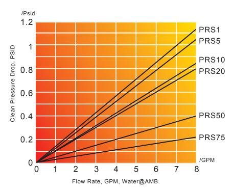
Flow rate is per 10" cartridge. For liquids other than water, multiply the pressure drop by the fluid viscosity in centipoises
