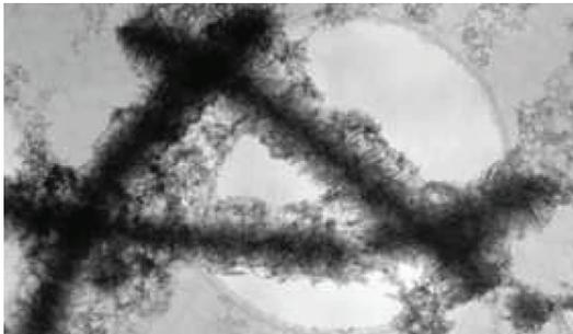
*Fig. 1: Shown above are three, 0.65 micron microglass fibers coated with alumina that form a pore approx 3 x 2 microns in size. Such a large pore allows for high flow rate at very low pressure drop but as a mechanical filter, has only about 2-3 micron initial efficiency. There are approximately 400 such pore structure layers in the ULTRA-D filter media to produce an excellent depth filtration media.*
